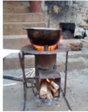
Fig. 3.12: Used as Rocket Stove
