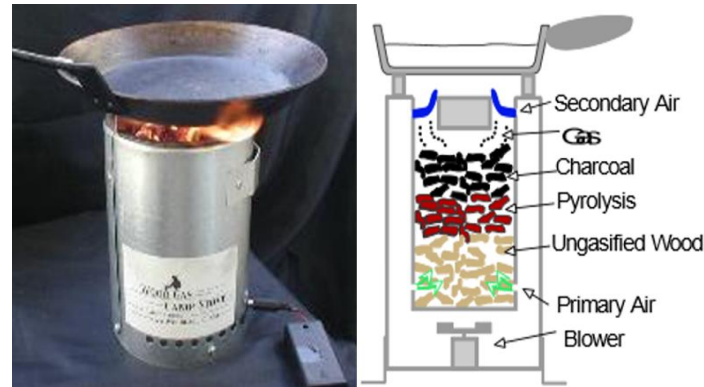
Figure 2.5: Left, 3-D view of a TLUD Stove in Operation; Right, factors involved in the Process
